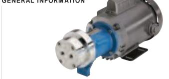
Liquiflo's **4-Series** pumps are low-flow magnetically-driven external gear pumps that are completely field repairable. The 4-Series housings are manufactured from Bar Stock in **316 Stainless Steel**, **Alloy-C** or **Titanium**. With several material options for shafts, gears, wear plates and bearings, these pumps can be used in a wide variety of chemical processing applications.
