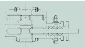
FIG.1 PACKING SEAL
