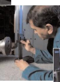
Technicians measuring the dimensions of pump components with precision calipers: Liquiflo pump components are precisely manufactured to tolerances as low as .0004 inches (10 microns).
