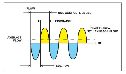
Upper (yellow) graph shows flow rate as function of time for a reciprocating diaphragm metering pump. The diaphragm pump produces large pulsations and high instantaneous flow rates. These pulsations are detrimental to precise metering and cause the diaphragm pump to require more suction pressure to operate effectively. Rotary gear pumps produce a smooth, pulseless flow (dashed line) and require less NPSH, making them ideal for metering applications.
