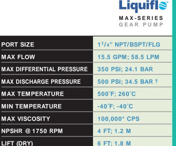
WEIGHT (without motor)SEALED, Close-CoupledMAG-DRIVE, Close-Coupled55.5 LBS; 25.2 KGS55.5 LBS; 25.2 KGS
