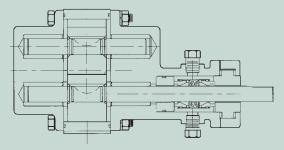
FIG.4 DOUBLE MECHANICAL SEAL
